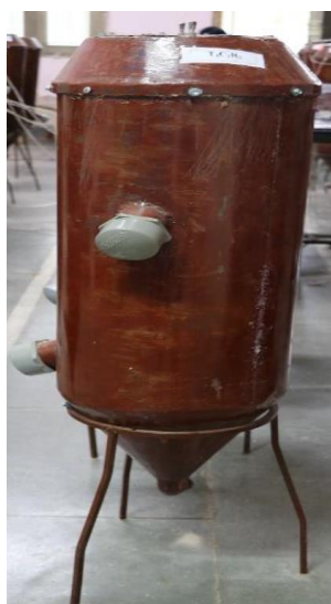
Plate 5.1. Fabrication of storage bin specifically designed with ozone gas circulating system
